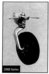
"Standard bracket is for 1 1/2 " leafspring. If required for use with 1 1/4" leafspring, use P/N 1478-00 spacer and P/N 1306-00 adapter.
