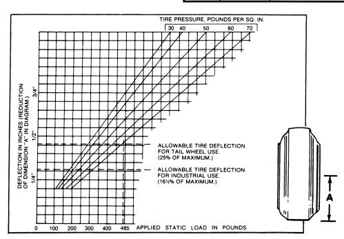
Tire deflection under load (shown as reduction of dimension "A") as load is applied using a given tire pressure (see chart).
