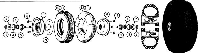
The Model 2600 is used on all Scott tailwheel applications requiring an 8" diameter tire. Available for general use, it is also suggested for helicopters, liaison and primary training aircraft, and material handling devices where low weight and high strength are required.
